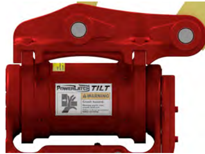
Fig 4.10 Position of warning notices
